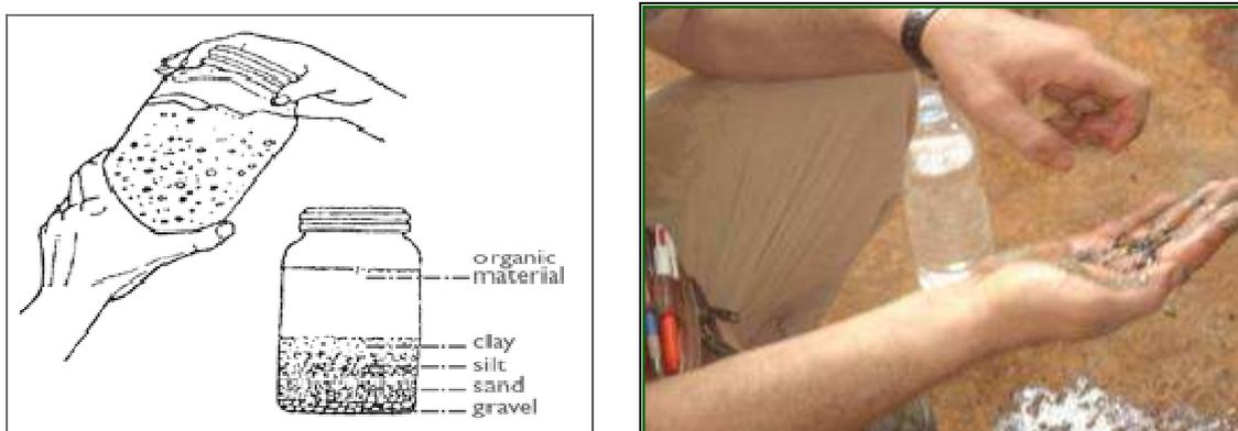
Figure 9 sedimentation test carried at Morang district
